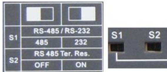
Figure 2.10 S1 and S2 switch position
