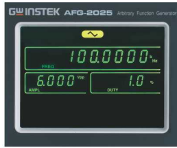
1% Duty Cycle of Square Wave Setting
